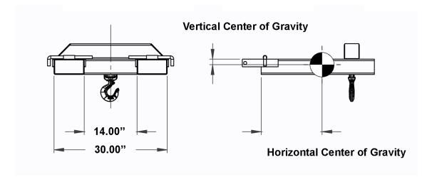
Model = MFSH-10 Empty Weight = 142 lbs Vertical Center of Gravity = 1.45" Horizontal Center of Gravity = 16.13"
