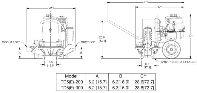
\*\*This dimension may vary due to engine manufacturer's specifications. NOTE: Dimensions are in inches (centimeters) and have a tolerance of +- 1/8".
